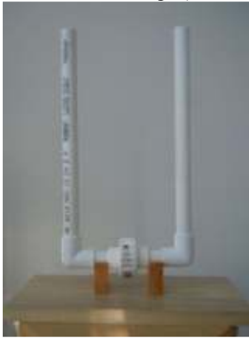
Figure 3: The first prototype was constructed by connecting a long pipe, a slip elbow, a short piece, a union, a short piece, a slip elbow and a long piece of ½" inner diameter PVC piping.
