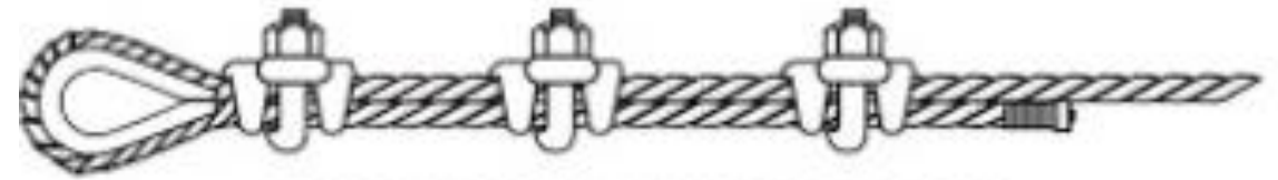
RIGHT WAY FOR MAXIMUM ROPE STRESS
