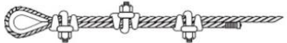
WRONG WAY: CLIPS STAGGERED
