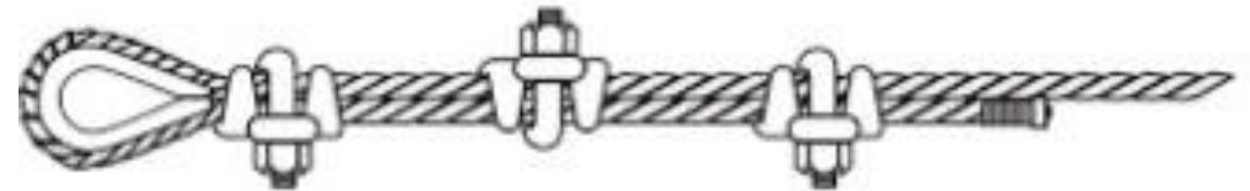
WRONG WAY: CLIPS STAGGERED
