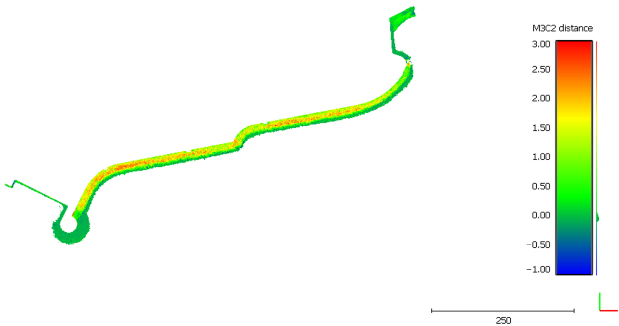
Figure 10. Comparison between DSM 1 (reference) and DSM 2 (compared) on the emerged breakwater, with distance values limited within the interval (-1; 3) m.
