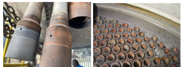
Figure 11: Extreme low liquid level on top tube-sheet, visible as color change.
