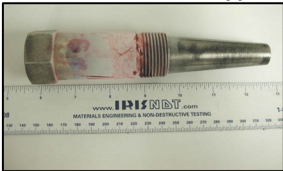
Figure 11. Penetrant Testing (PT) of thermowell with chloride stress corrosion cracking.
