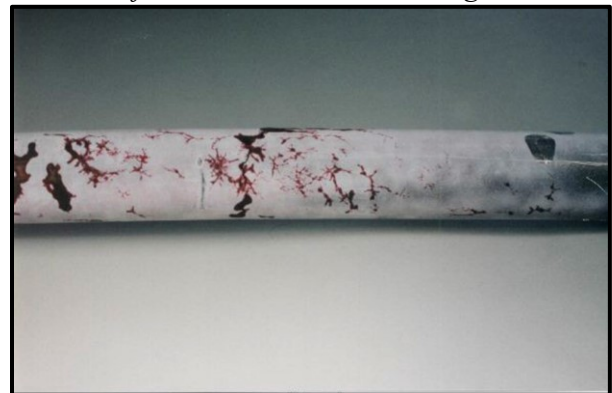
Figure 2. Color contrast PT results
