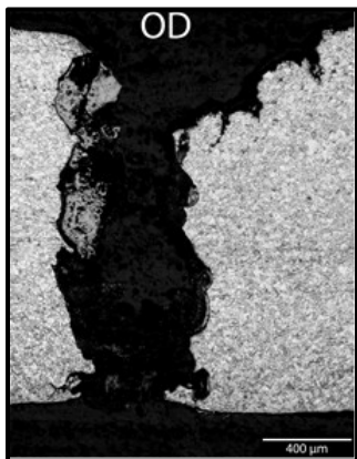
Figure 15. The CP-Ti tube pits are steep, narrow, and tend to tunnel. Kroll's Reagent Etch.
