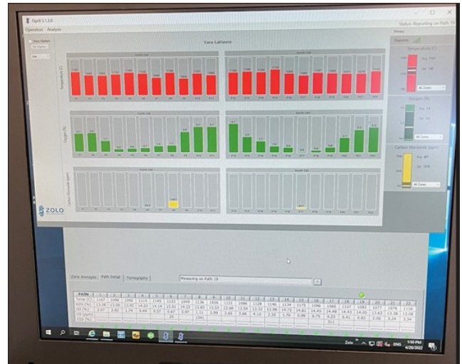
Figure 11. ZoloSCAN™ TDLAS raw data output, showing temperature (top, red), oxygen content (middle, green) and carbon monoxide content (bottom, yellow) for each sub-cell.
