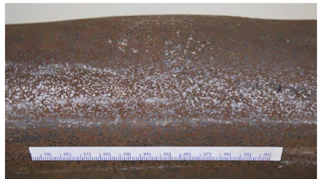
Figure 4: Bulging evident on the failed tube
