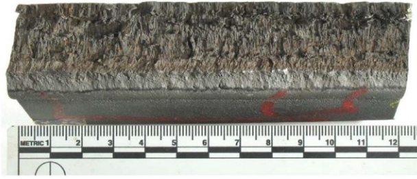
Figure 8, Specimen taken along fracture surface on the longitudinal weld seam
