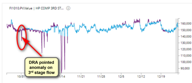
Figure 3. Flow detection by DRA
