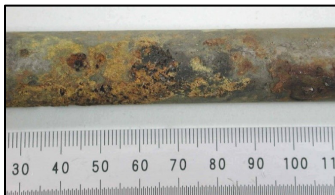
Figure 4. Type 304L stainless steel condenser tube with pits and cracks.
