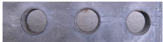
Figure 5. Effect of nitriding in a perforated plate operated for 20 years
