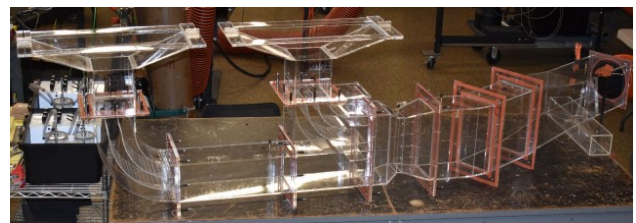
Figure 2: 1:12.5 scale model of the convection section outlet duct used for modeling of the custom venturi
