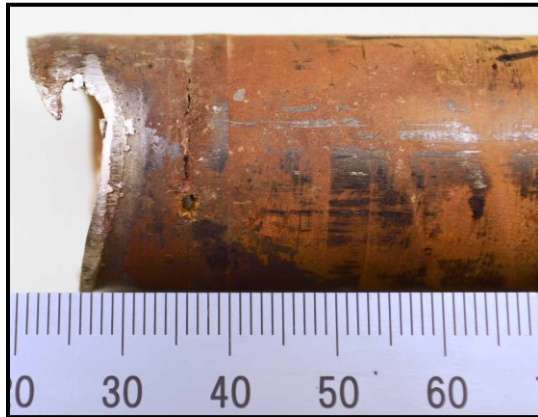
Figure 14. CP-Ti tube OD surface with through wall holes and bright orange scale.
