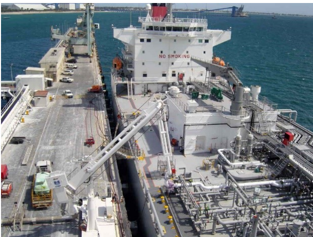
Figure 2. Ammonia import line connection
