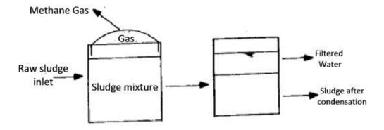
Fig (2-17): Two stages anaerobic sludge digester
