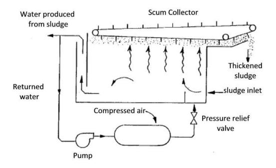
Fig (2-14): Air Floatation Sludge Thickeners
