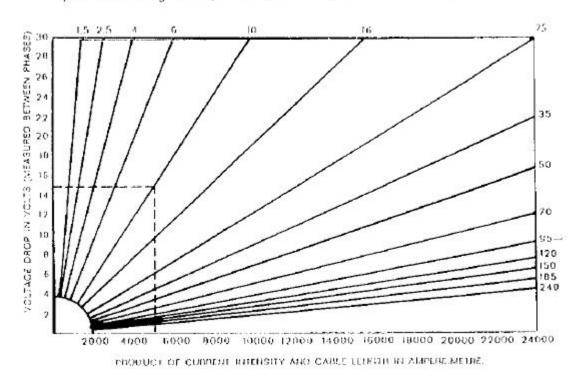
Fig (2-30): Nomogram for calculation of voltage drop for 3- core cable, 3- phase alternating current,  $\cos \phi = 0.8$
