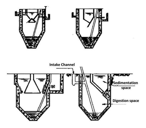
Fig (2-6): Horizontal flow sedimentation tanks (IMHOFF Tanks)
