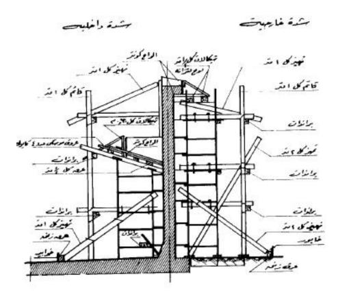
Fig (3-6): Formworks of a weir give fair face
