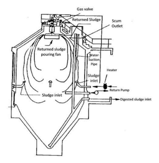
Fig (2-16): High rate sludge digester components
