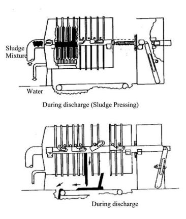
Fig (2-22): Sludge Filter Press
