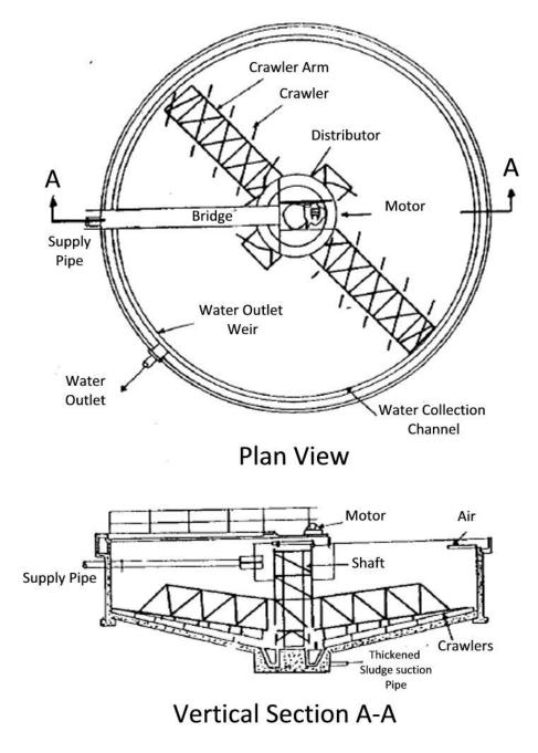
Fig (2-13): Mechanical Sludge Thickeners
