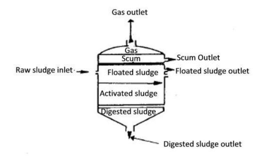
Fig (2-15): Conventional Sludge Digester
