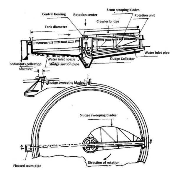
Fig (2-5): Horizontal flow circular sedimentation tanks
