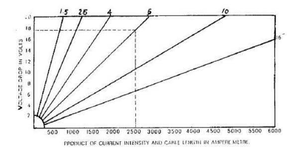
Fig (2-29): Nomogram for calculation of voltage drop for double cores cable, single phase alternating current,  $\cos \phi = 1.0$
