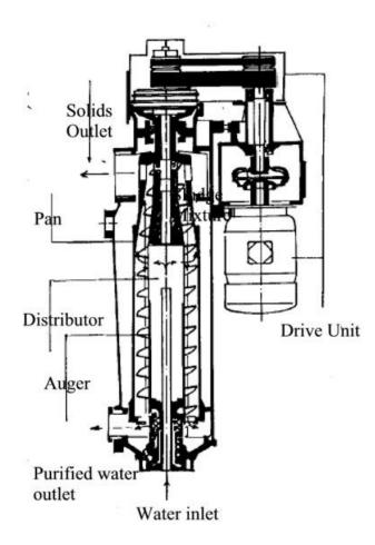
Fig (2-23): Sludge thickening systems using centrifugal forces
