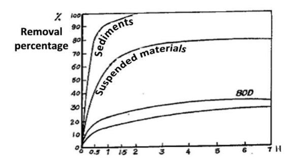
Fig (2-7): Removal percentage of sediments, suspended materials and organic materials in sedimentation tanks
