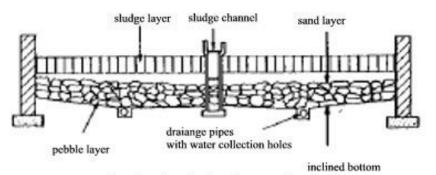
Section in sludge dewatering bed
