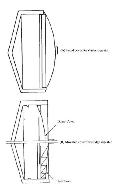
Fig (2-18): Foxed and movable cover of sludge digester
