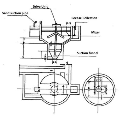
Fig (2-3): Circular sand separation bed
