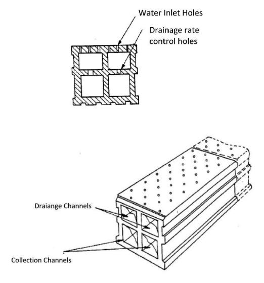
Fig (2-10): Drainage Channels
