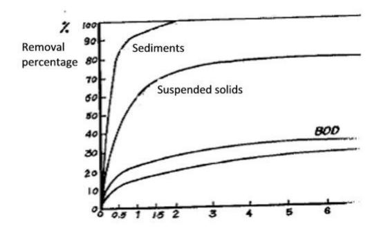
Fig (1-3): Removal percentage of sediments, suspended materials and organic materials in sedimentation tanks
