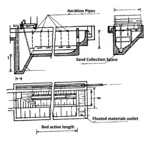
Fig (2-4): Rectangular aerated sand separation bed
