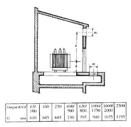
Fig (2-28): Installation of transformers in sealed enclosure
