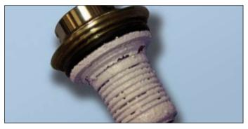
Fig. 5.7: Metal bellows seal clogged by lime scale build-up
