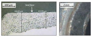
Fig. 5.9: Selective corrosion in cemented tungsten carbide. The metallic binder phase is corroded resulting in reduced wear resistance
