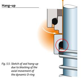
Hang-up of a mechanical shaft seal means that the axial movement of the rotating part of the shaft seal is blocked. Hang-up mainly occurs in connection with O-ring-type seals, but is also seen in connection with bellows seals, although the underlying mechanism is different.
