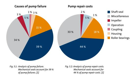
Typical shaft seal failures depend highly on the seal type and material pairing. O-ring-type shaft seals with dynamic O-ring and one seal ring in carbon-graphite typically have problems with wear on seal faces and seal hang-up, which prevents axial movement of the dynamic O-ring and seal ring. Mechanical shaft seals with hard/hard seal face material pairings usually experience problems associated with dry running.
