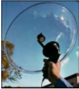
Parabolic dish used with ultrasonic detector greatly extends detection range abilities.
