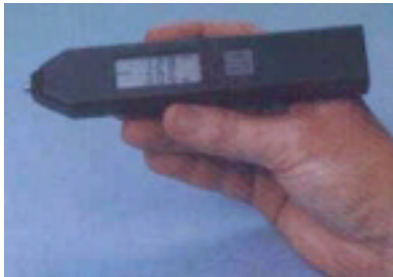
Examples of typical handheld vibration sensing meters. Note readout providing immediate level indication.
