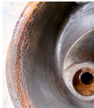
Figure 11: Cavitation damage on the suction side of the blade that has been worsened in a corrosive and erosive environment.
