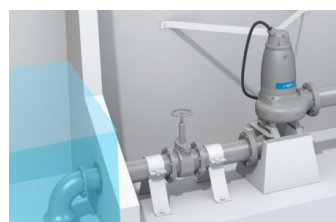
Figure 15: A dry-installation including a bell-shaped suction inlet, a gate valve, a suction elbow (180°) and a pump.
