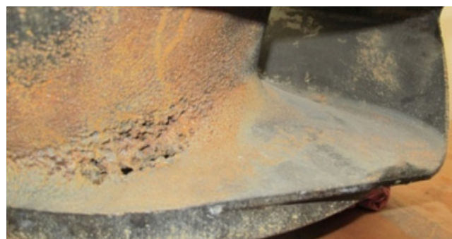
Figure 22: Cavitation damage on the pressure side caused by clogging
