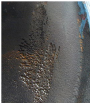
Figure 10: Damage from sheet cavitation on the suction side near the leading edge of an impeller blade.
