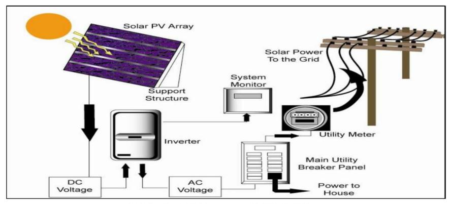
**Grid-Tied PV System (ON-GRID)**
