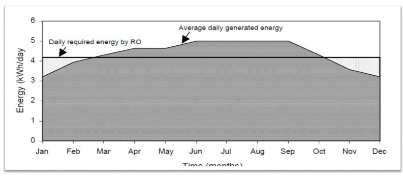
Figure 3 The average daily generated energy versus that required by the RO unit at different months
