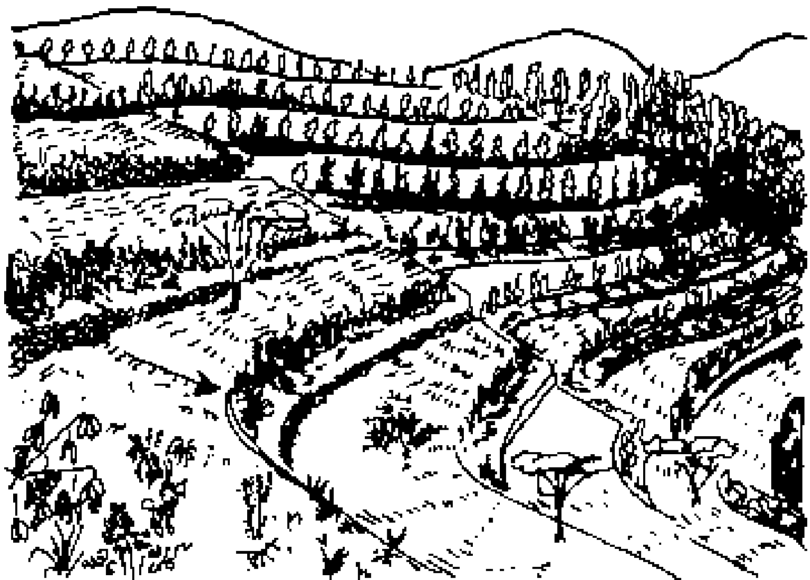
Figure 38. Contour bench terrace for water harvesting.
