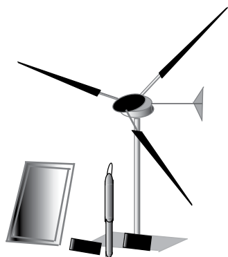
Figure 22. Combination of solar and wind-powered pumps.
