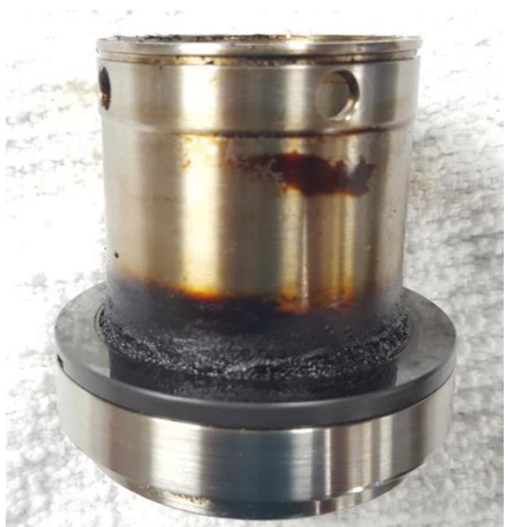
Severe heat damage done by dry running of the seal. Process coking on the sleeve between primary seal and mating seal face.
