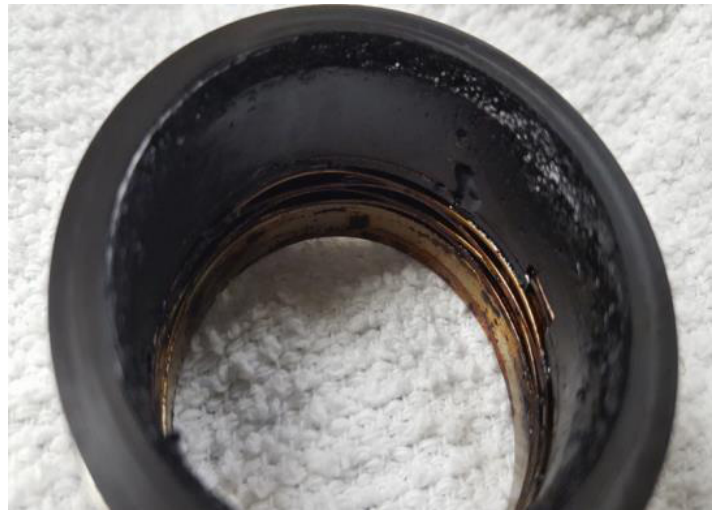
Damage to seal face due to dry running, plus mechanical distortion.
