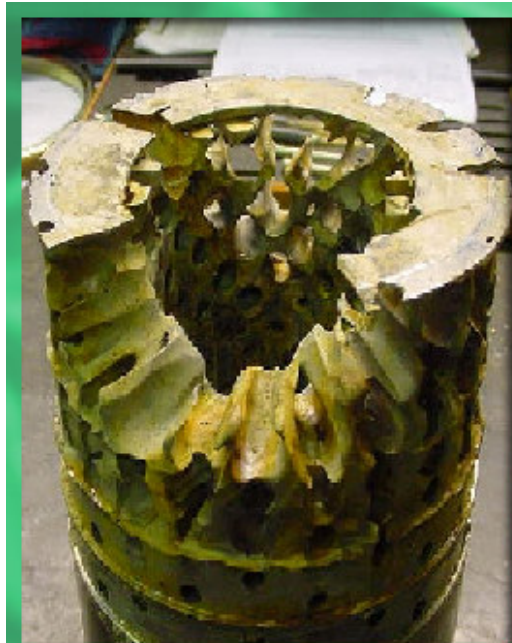
Erosion Caused by Sand
