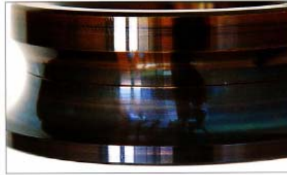
Photo 7-18-2 Part: Inner ring of a 4-point contact ball bearing Symptom: Bluish or purplish discoloration on raceway surface Cause: Heat generation due to poor lubrication
