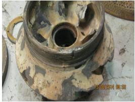
• Sometimes the impeller is disintegrated into two pieces.
