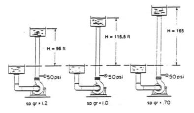
Three pumps designed for same pressure will develop heads (ft. of liquid) inversely proportional to the specific gravity.
