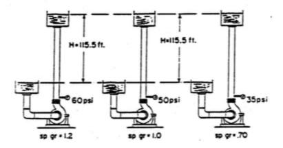
Three identical pump, each designed to develop 115.5 ft. of head (water Sp. Gr. 1.0) when liquids of other Sp. Gr. are handled, the head (in feet) will remain the same, but the pressure will very proportional to the specific gravity
