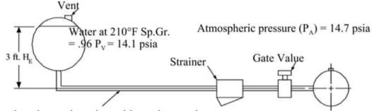
Friction loss in suction pipe with strainer and gate valve  $H_F = 1\frac{1}{2}$  ft.
