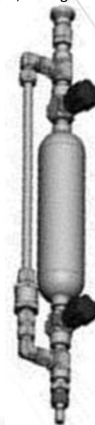
Cylinder with bypass to flushing the quick connectors
