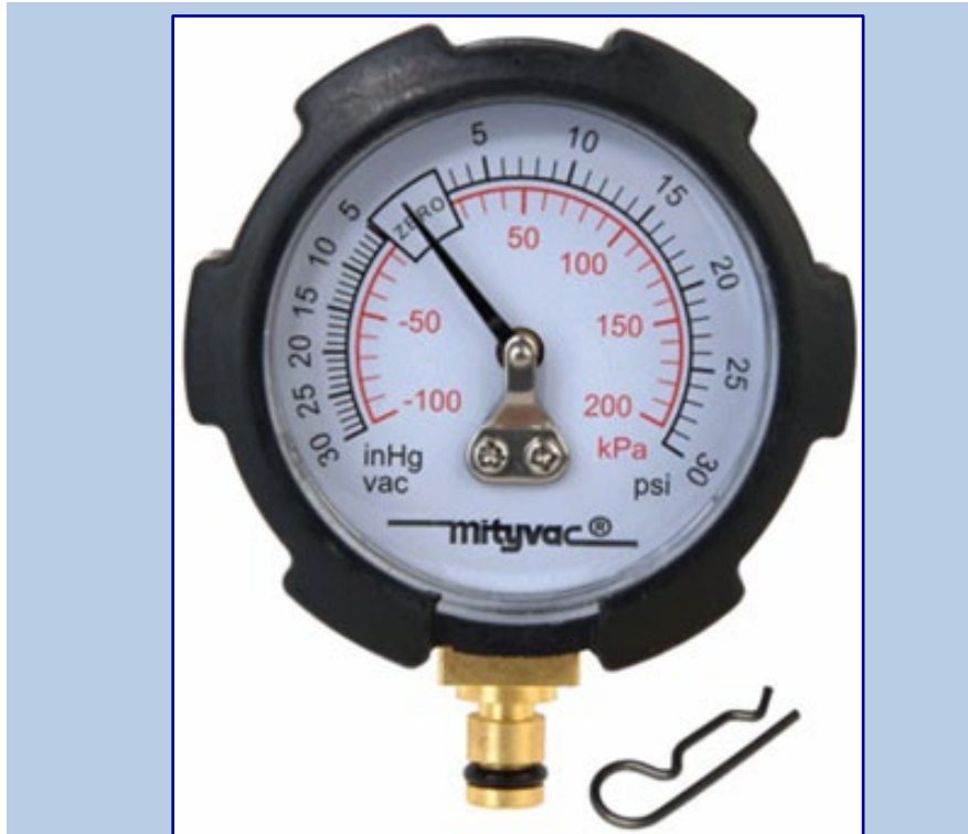
Typical compound Suction pressure Gauge.
