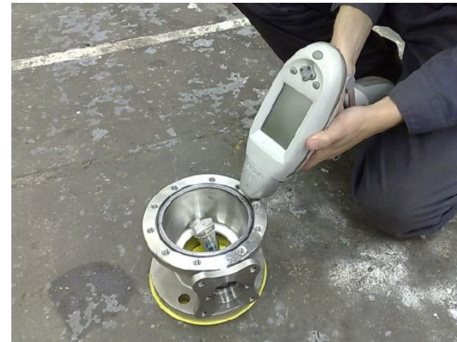
Example of testing with hand-held XRF analyzer www.iimtiruchy.org
