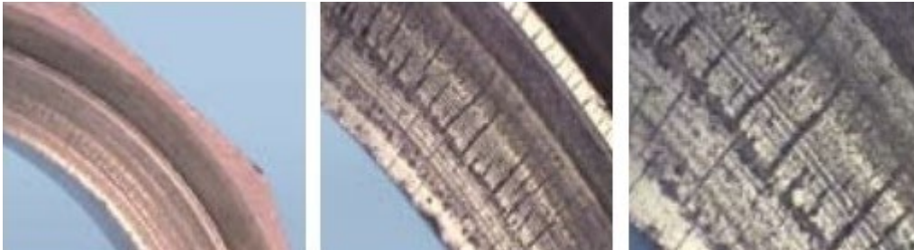
Thermal cracks in seal face caused by poor lubrication
