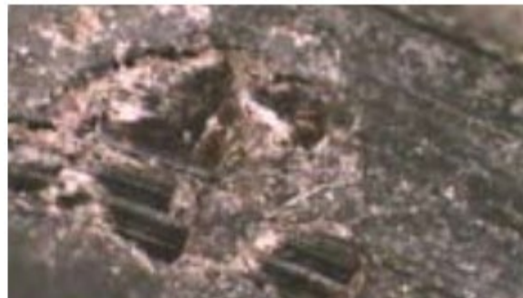
Surface damage due to high temperature on EPDM and FKM secondary seals
