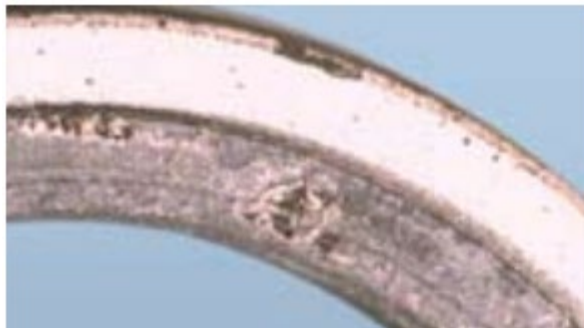
Deposits on carbon graphite seal face
