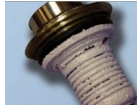
Metal bellows seal clogged by lime scale build-up
