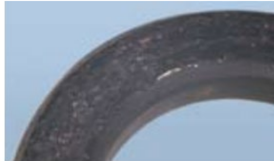
Surface damage due to high temperature on EPDM and FKM secondary seals
