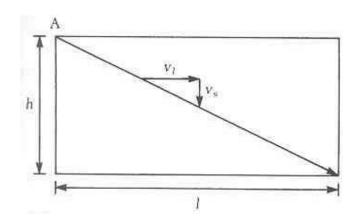
This trajectory represents a particle which has a settling velocity  $v_0$
