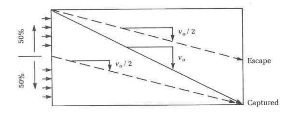
v<sub>0</sub> expressed in units of flow per unit area is called the **Overflow rate**
