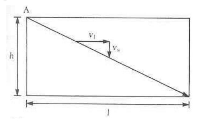
$V_s$  = settling velocity of the particle  $V_l$  = horizontal velocity of liquid flow
