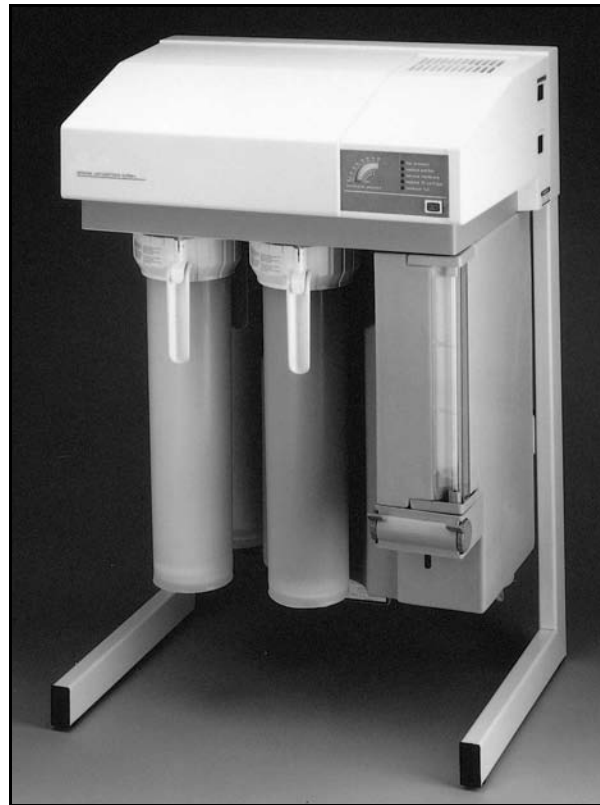
Figure 1-50 Reverse osmosis system with cartridge polisher
