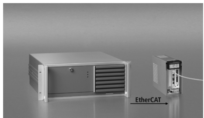
Figure 8: EtherCAT leads to smaller controllers
