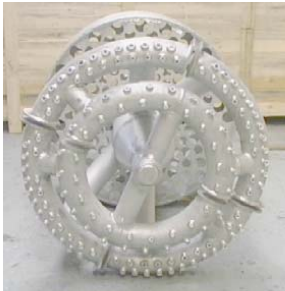
Figure 11. Johnson Matthey Catalysts burner gun
