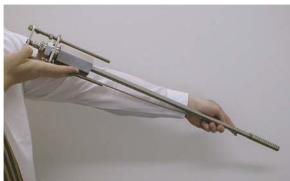
Figure 14. TRACERCO catalyst probe
