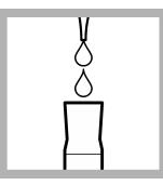
6. Prepared sample: Use a plastic dropper to add 0.5 mL of cyclohexanone to the solution in the mixing cylinder.
