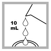
**5. Blank preparation:** Pour 10 mL of the solution into a sample cell.
