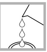
**10.** Pour the prepared sample solution from the mixing cylinder into a second sample cell.
