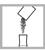
**3.** Add the contents of one ZincoVer 5 Reagent Powder Pillow to the mixing cylinder. Close the cylinder.
