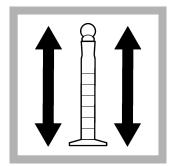
**4.** Shake the cylinder vigorously to dissolve the powder completely. Inconsistent readings can result if all the particles are not dissolved.
