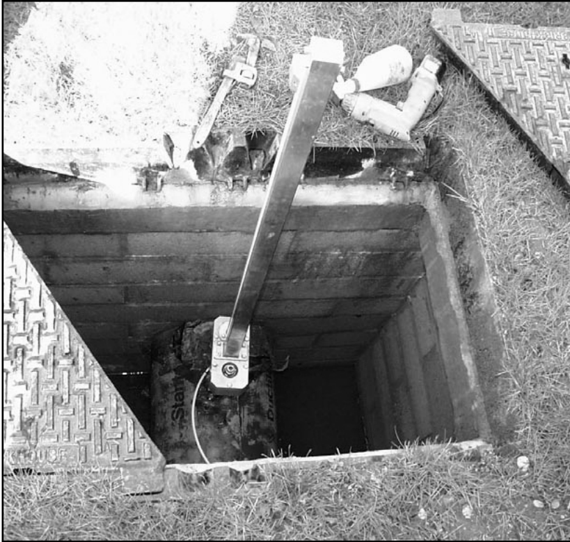
Figure 1 The trunk mains sampler in position on a trunk main
