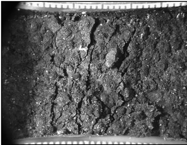
Figure 3 Corrosion scale from galvanized pipe coupon at 10\times magnification (wet condition)
