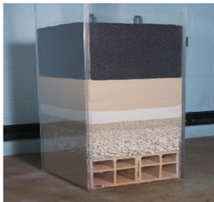
Water passes through charcoal, sand, and gravel layers in a water system's filtration tank.
