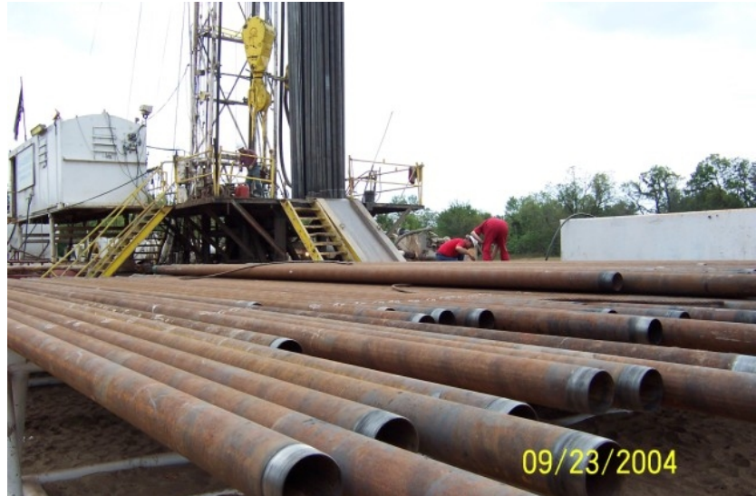
Figure 49 Casing Ready To Run
