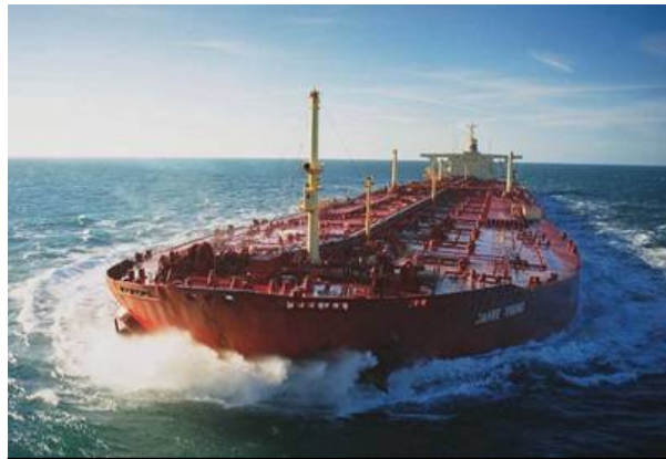
Figure 117 - Super Tanker Jahre Viking. This tanker can carry 564,700 tonnes crude oil; it would take the Alyaska pipeline 4 days to fill this tanker. It has been converted to an FSO (Floating Storage and Offloading) vessel.
