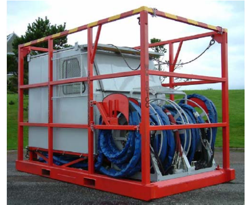
Figure 98 CTU Control Cabin
