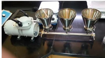
-Membrane filtration equipment.
