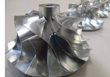
Figure 3. full length splitter impeller
