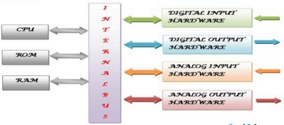
The LCU receives inputs from measuring devices and commands from operators and computes the control output needed to make the process follow the commands. It then sends the outputs to the actuators, drives, pumps, valves and other mechanical devices that regulate the process in field. The CPU does this process and it communicates with all the devices in LCU through the internal bus, which transmits addressing, data control and status information in addition to the data.
