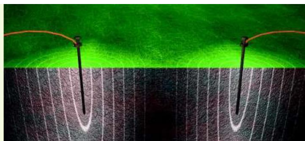
Figure 34: Spheres of Multiple Earth Electrodes
