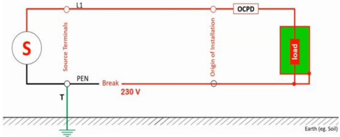
Figure 13: Neutral breakage in TN-C System
