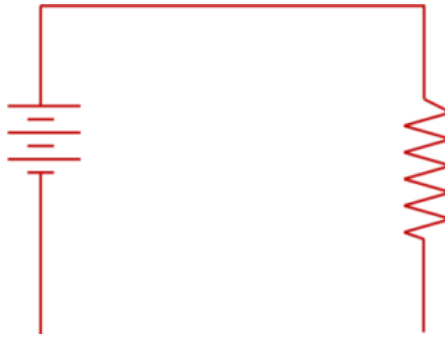
Figure 41: Incomplete circuit or open circuit, no current will flow in above condition.
