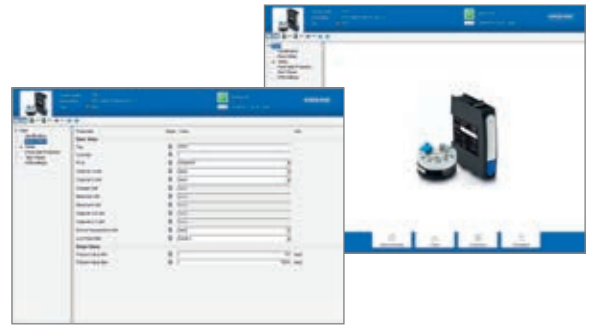
Configuration of OPTITEMP TT 51 temperature transmitter via PACTware™
