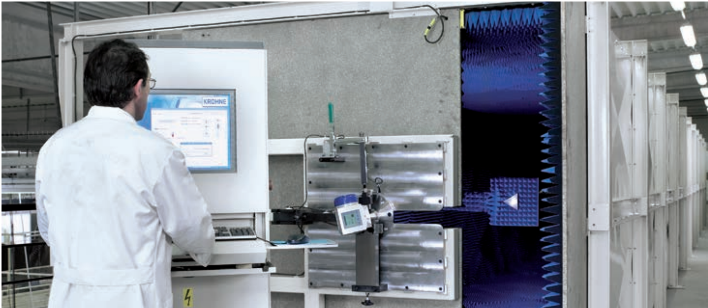
Calibration rig for FMCW level transmitters
