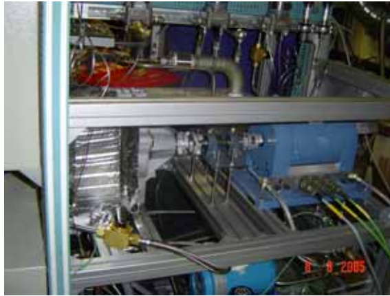
Figure 3.42 – Turbine and eddy current brake coupling.
