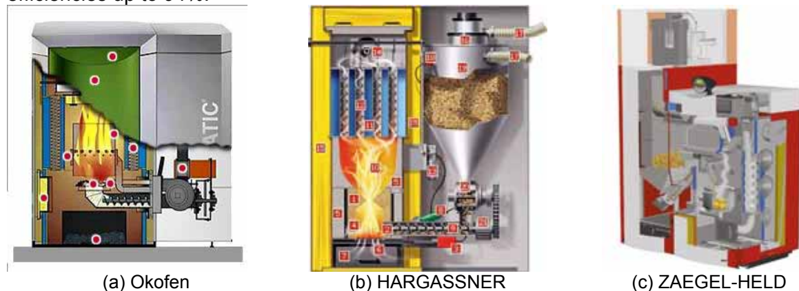
Figure 3.2 – Types of pellets burners by there feed principle: (a) Bottom fed burner; (b) horizontal fed burner; (c) top fed burner.
