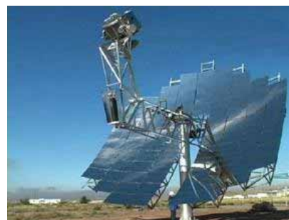
Figure 3.14 – Parabolic dish reflector [MIL04].
