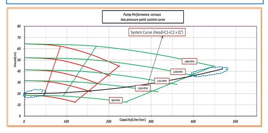
Pump Performance curve for two Duty pumps operation
