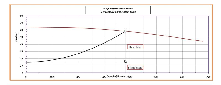
H=Static Head +Frictional Head Loss H=Constant1+Constant2 xQ<sup>2</sup>
