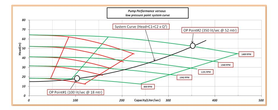
$$\begin{array}{ccc} H=C1+C2xQ^{2} \\ 18=C1+C2x(0.1)^{2} \\ 52=C1+C2x(0.35)^{2} \\ C1=15 & \& & C2=302.2 \\ H=15+302.2xQ^{2} & & 10 \end{array}$$
