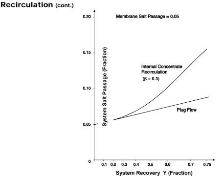
When the recirculated concentrate stream approaches zero, the  $\beta$  number approaches 1/[(1/Y) –1], and the recirculation system becomes a plug flow system. A compromise between plug flow and recirculation systems is the tapered recirculation system with a declining number of parallel modules per stage when viewed in feed flow direction (see Figure 3.8).
