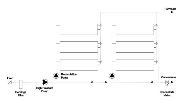
The main advantage of the recirculation concept is the defined feed flow rate to the modules regardless of the degree of fouling of preceding modules and the changes in feed water composition. Further aspects of the recirculation concept are mentioned in <u>Batch vs.</u> <u>Continuous Process (Section 3.2)</u>, and <u>Single-Module System (Section 3.3)</u>. A comparative summary is given in Table 3.3.
