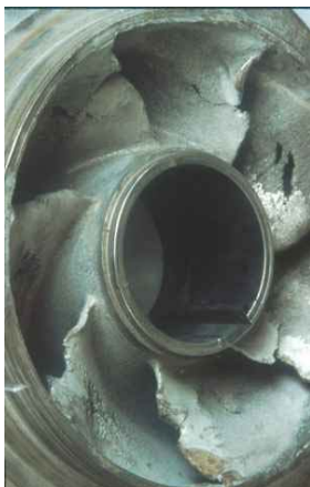
Figure 166: cavitation phenomenon relating to centrifuge pump blades
