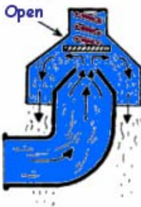
Figure 164: equipment to protect against overpressure
