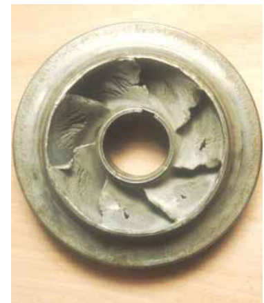
Figure 166: cavitation phenomenon relating to centrifuge pump blades
