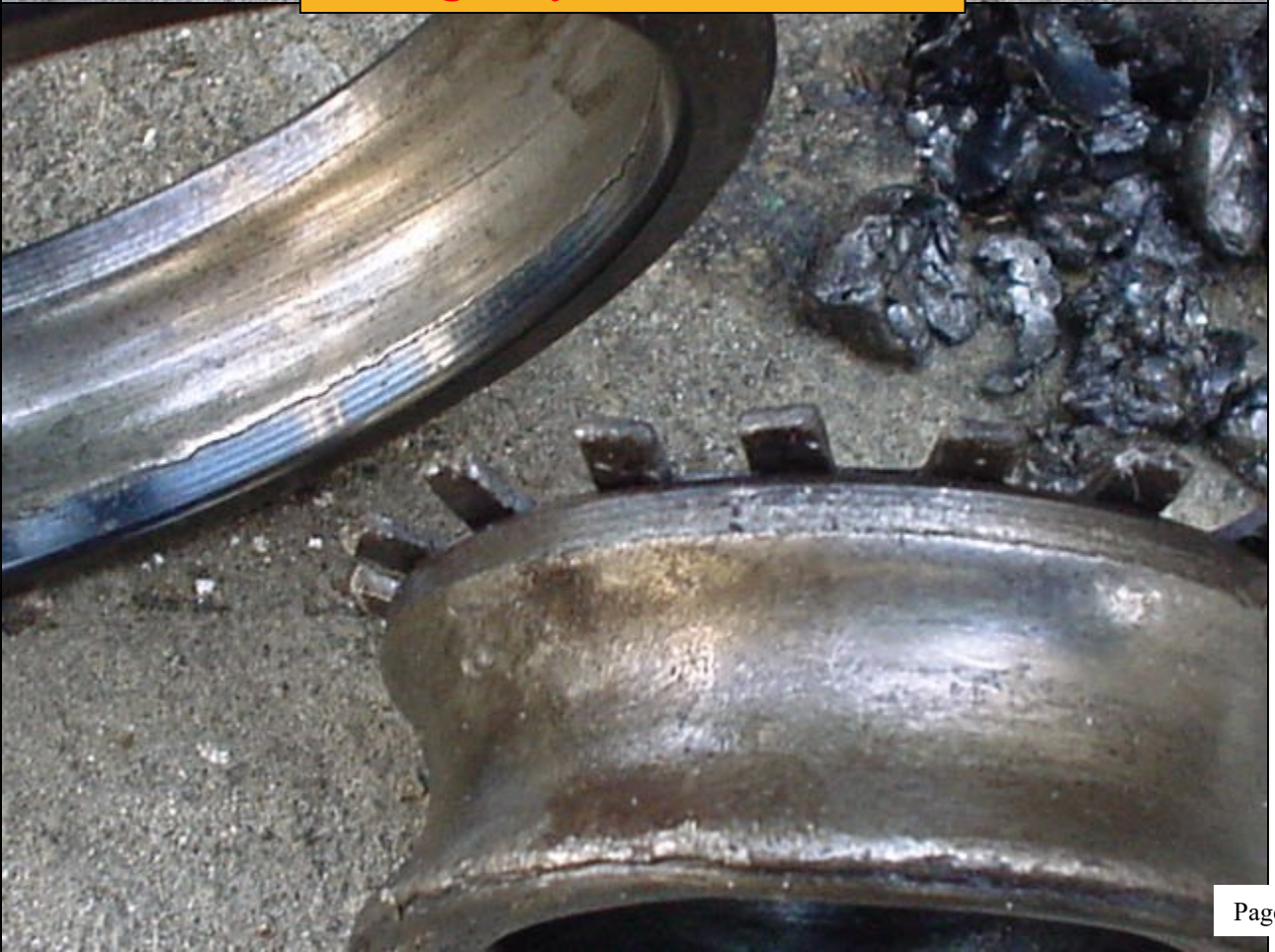
Pure Mist Lubricated Bearing Damaged by loss of Mist
