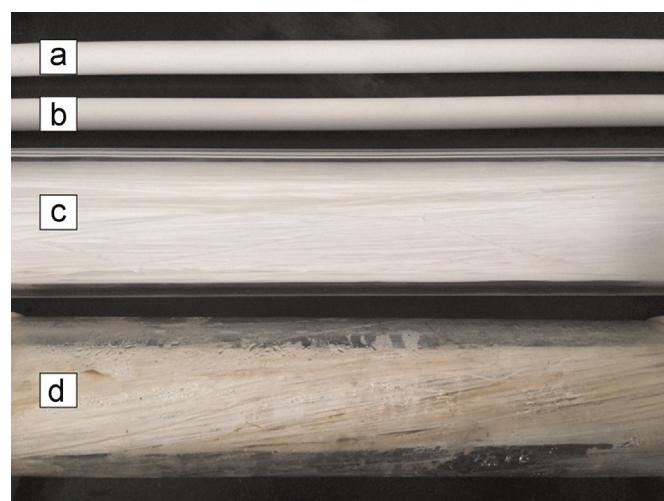
Fig. 17. Images of (a) fresh SC membrane, (b) SC membrane after one month on site operation, (c) fresh PP hollow fiber membranes and (d) PP membranes after one month on site operation.
