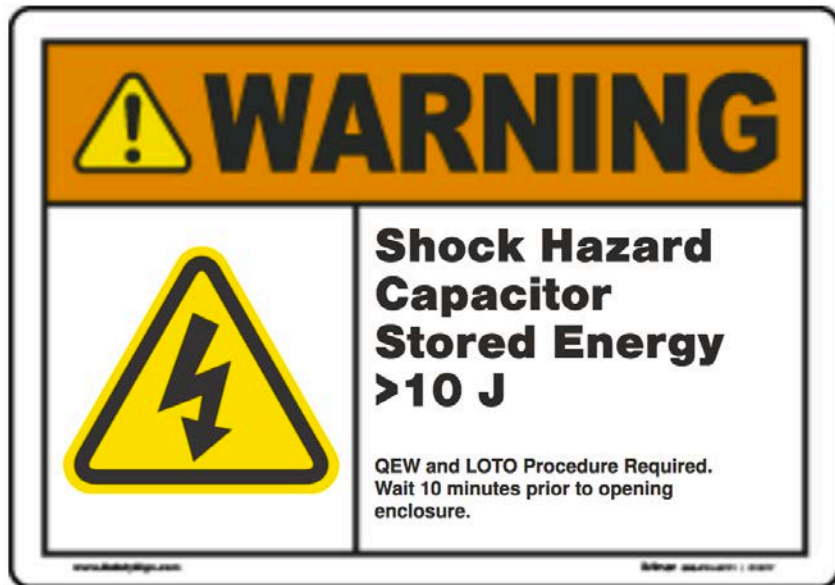
Fig. 15.6.1 – Example of a capacitor stored energy warning label
