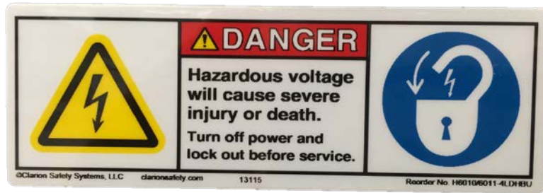
Fig. 5.3.3.a – Example of label applied to hard-wired equipment, indicating requirement to lock out prior to servicing.
