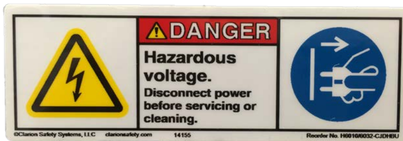
Fig. 5.3.3.b – Example of label applied to cord-and-plug equipment, indicating requirement to unplug prior to servicing.
