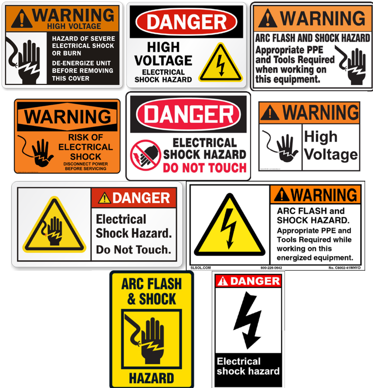
Fig. 5.3.2.c– Typical Hazard Warning Labels Found on Electrical Equipment
