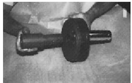
Picture 15: Installing Permeate Port 6
