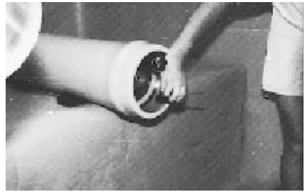
Picture 6: Tapping Securing Ring 11 into Position
