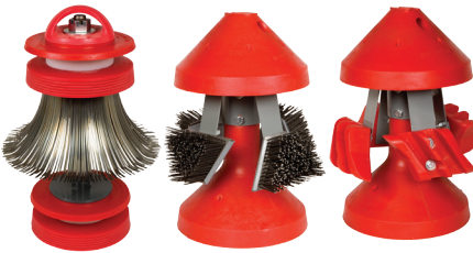
Fig 98. Pigs with Blades and Brushes Standing on End
