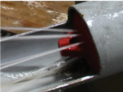
Fig 62. Debris Suspended in Front of the Pig
