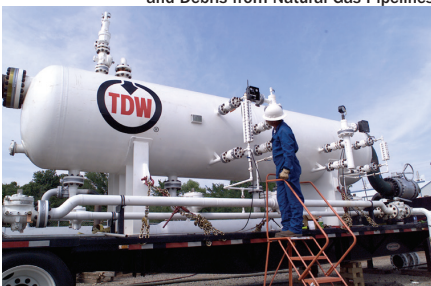
Fig 46. Portable Separator - to Remove Liquids and Debris from Natural Gas Pipelines
