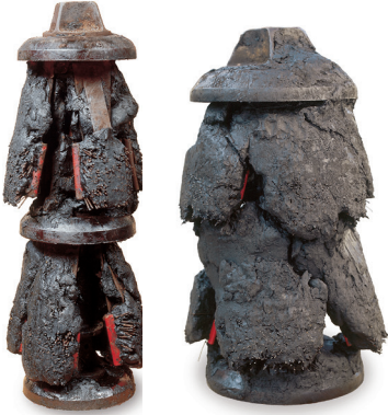
Fig 96. Cleaning Pigs Packed with Paraffin
