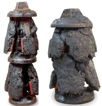
Fig 65. Cleaning Pigs Packed with Paraffin
