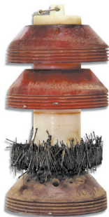
Fig 45. Pig with Magnets to Collect Debris
