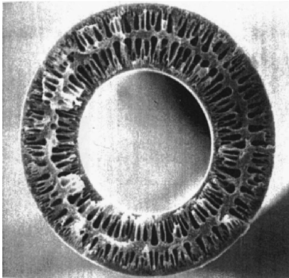
Hollow fiber cross section of  $\varnothing \approx 1$  mm
