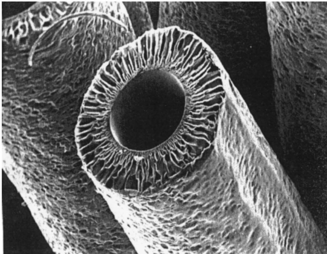
Hollow fiber made of polysulfone
