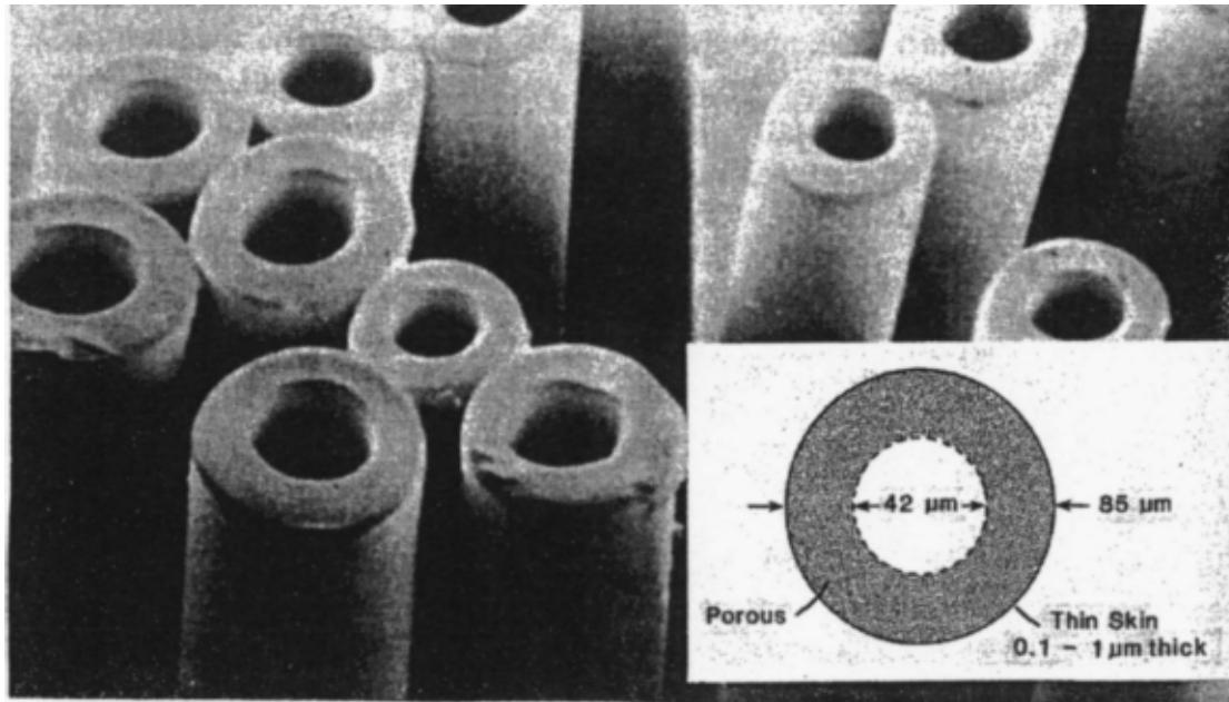
Hollow fiber cross section of polyamide
