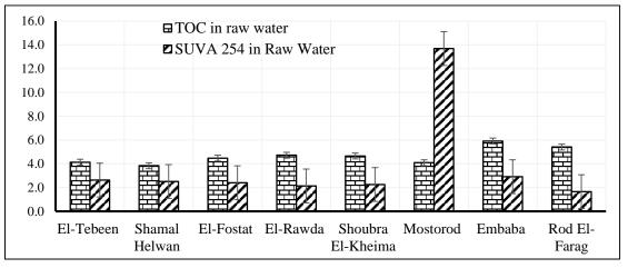
Figure 1: TOC (mg/l) and SUVA<sub>254</sub> (L/mg. m) in raw water
