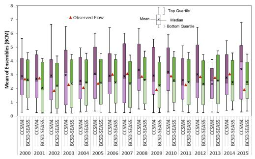
Figure 1. 10 days boxplot of the mean ensemble of forecasted flow and the mean of observed flow for the LT6 at Diem station
