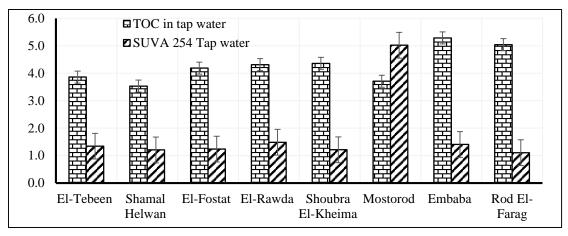
Figure 2: TOC (mg/l) and SUVA254 (L/mg. m) in tap water
