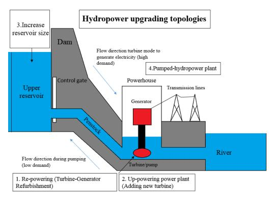
Figure 1: Hydropower upgrading topologies
