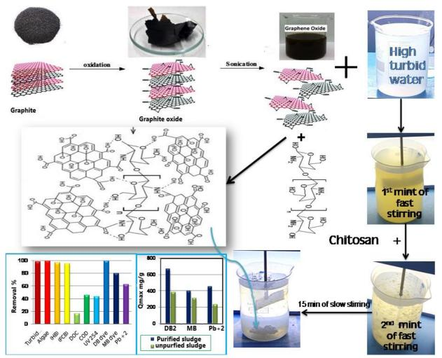
Figure 1: Graphical abstract shows the diverse steps during coagulation/flocculation process by GO/CS up to the last minute of the process beside its impact on various pollutants. Considering the economic aspect, the sludge generated during the coagulation/flocculation process has been effectively utilized as an adsorbent for further removal of dyes and Pb (II)
