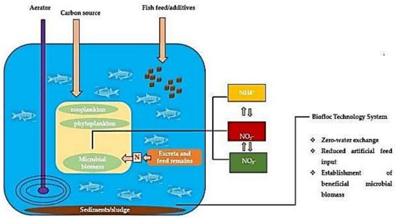
Figure 1. Schematic diagram of a biofloc technology system
