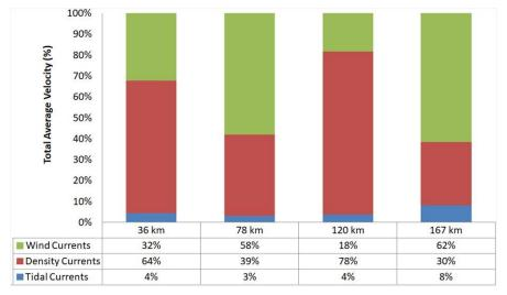
Figure 2. Extracted model total average velocity participation percentage over 200m depth at different locations along the basin of three current components at selected random time. Note station 0.0 is at the basin northern tip location.
