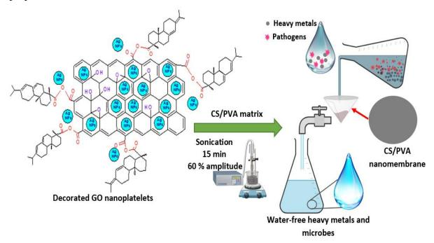
Figure 1. Decorated GO nanoplatelets by antimicrobial natural rosin acids and Ag NPs as a novel biomaterial for boosting the properties of CS/PVA nanomembranes
