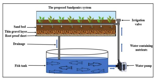
Figure 1. Schematic design of the experimental layout.
