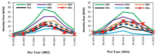
Figure 2. Probability of exceedance of the ensembles of the forecasted flow and the observed flow for the whole season at Diem station, straight lines present the performance of CCSM4, dotted lines present the BCSD-SEAS5
