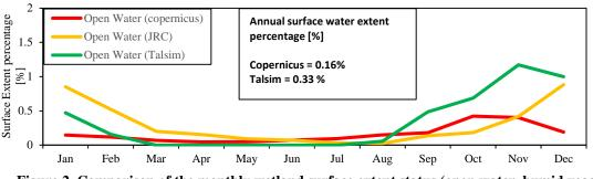
Figure 2. Comparison of the monthly wetland surface extent status (open water, humid vegetation) between TalsimNG and satellite processing images (Copernicus, JRC).
