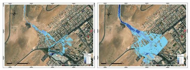
Figure 1. Flow depth output overlaid with a satellite image of the affected area for the no embankment condition (left). Maximum Flow Depths of the February 21, 2020 Event Reenactment (right)
