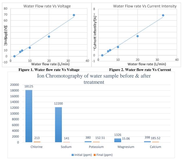
**Figure 3.** The initial and final concentration of real sea water samples after 10 days testing In conclusion, TENG stage is 30 % efficient than the traditional dynamo. The desalinated is valid for irrigation exhibits satisfactory performance for irrigation purposes, particularly for potato crops, meeting the requirements outlined by the FAO.
