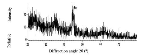
Fig. 2: The X-ray pattern of NZVI reveal an apparent peak at the diffraction angle 2θ value of 45°, which indicated the formation of Nano-iron in the Zerovalent state (Fe<sup>θ</sup>).
