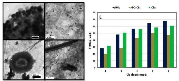
Figure 2: TEM images of GO after coagulation process show the synergetic effect of it on bacteria (A Wrapping, B perturbation of the cell membrane), TEM image of GO/CS binary system wrapping different contaminants during coagulation/flocculation process (C, D), the formation of TTHMs resulting from using different doses of chlorine in case of GO, GO/CS system and Chlorine dosing without coagulant (E).
