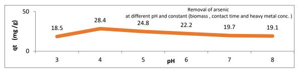
Fig. 1. Effect of pH on biosorption of arsenic by the dried microalgae *Chlamydomonas* sp. at constant time 60 min, biosorbent dose 1 gm/l, temperature 25 °C and heavy metal concentration 50 mg/l.
