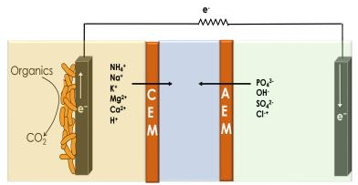
Figure 1. Schematic diagram of microbial nutrient recovery cell used in this study Table 1. Characteristics of sludge reject water used in this study (average ± standard deviation)
