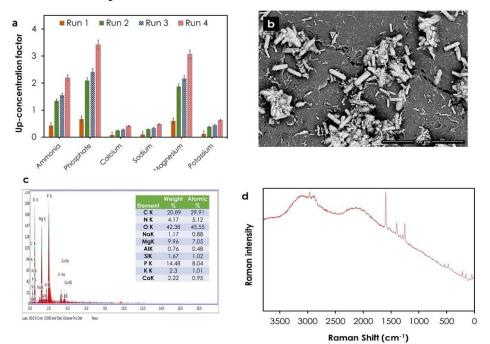
Figure 2. (a) Up-concentration factors for macronutrients at the end of six consecutive operational cycles for the MNRCs, (b) SEM image, (c) EDX spectra, and (d) Raman spectra of the crystal developed at the cathode surface of MNRCs.
