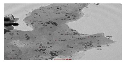
Fig. 1: TEM image of the synthesized NZVI particles, which have a nearly spherical shape with size range about (12-25) nm.
